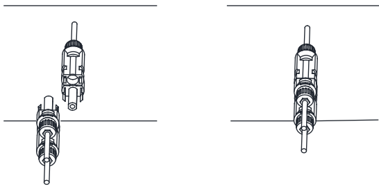
Pic 5.6 DC input connection
