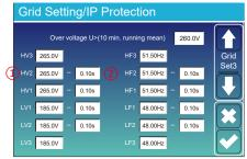
HV1: Level 1 overvoltage protection point;
