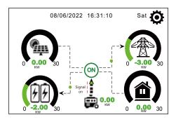
This page tells the PV and diesel generator power the load and battery.
