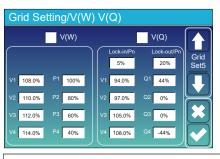
**V(W)**: It is used to adjust the inverter active power according to the set grid voltage.
