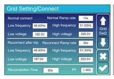
**Normal connect**: The allowed grid voltage/frequency range when the inverter first time connect to the grid. **Normal Ramp rate**: It is the startup power ramp.
