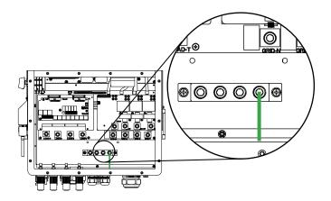
Earth connection(Copper wires)
