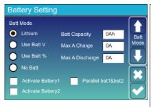
**Battery capacity:** it shows your battery bank size to Deve hybrid inverter.
