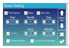
Factory Reset: Reset all parameters of the inverter. Lock out all changes: Enable this menu for setting parameters that require locking and cannot be set up. Before performing a successful factory reset and locking the systems, to keep all changes you need to type in a password to enable the setting.
