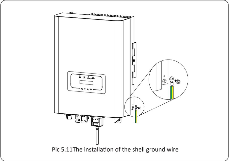
Pic 5.11 The installation of the shell ground wire
