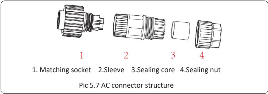
Step 3: Insert the cable (L1, L2, L3, N, PE) into the sealing sleeve.
